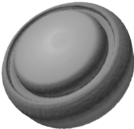
Figure 4: Battery, 3D-CT, outside view
