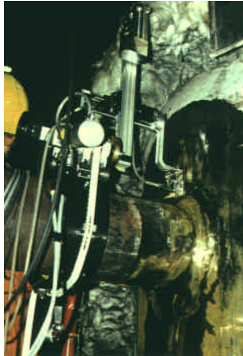
Figure 5: Automated Pre-heater Nozzle Examination
