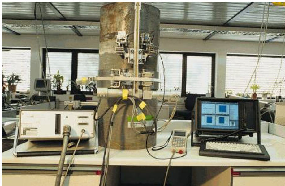
Figure 6: Portable PCUS 40 System w/ Pipe Scanner and Scanner Control
